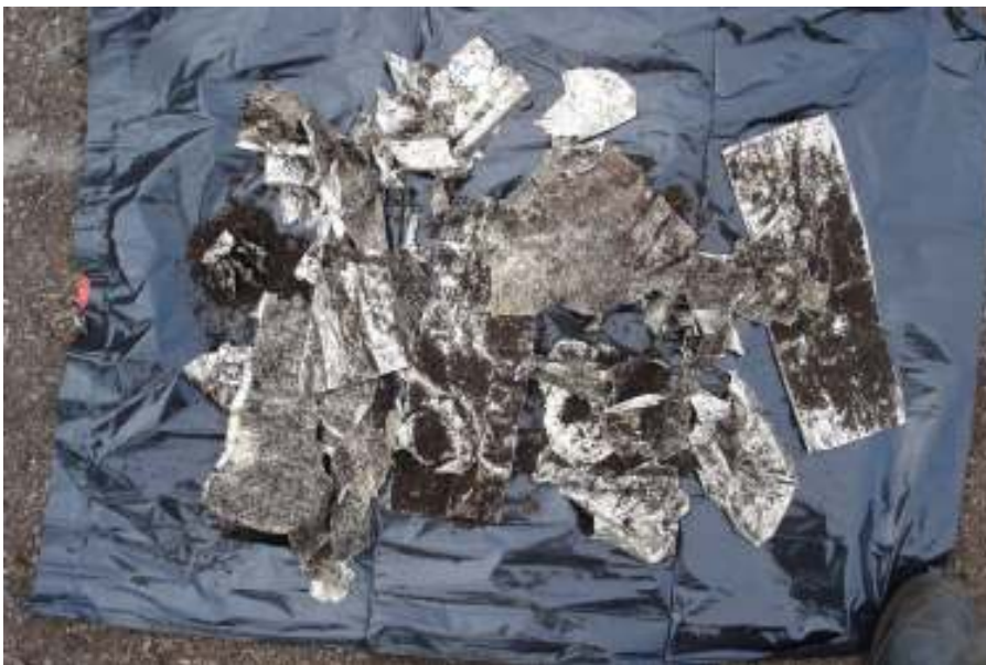
Bags fracturing upon contact
