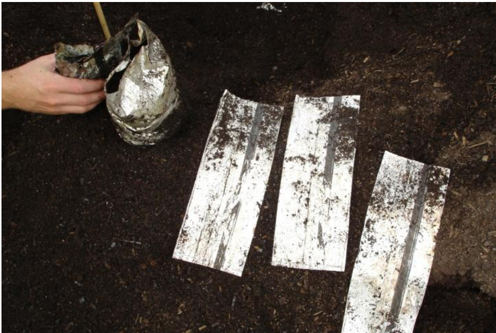
Filled bag tore on handling
