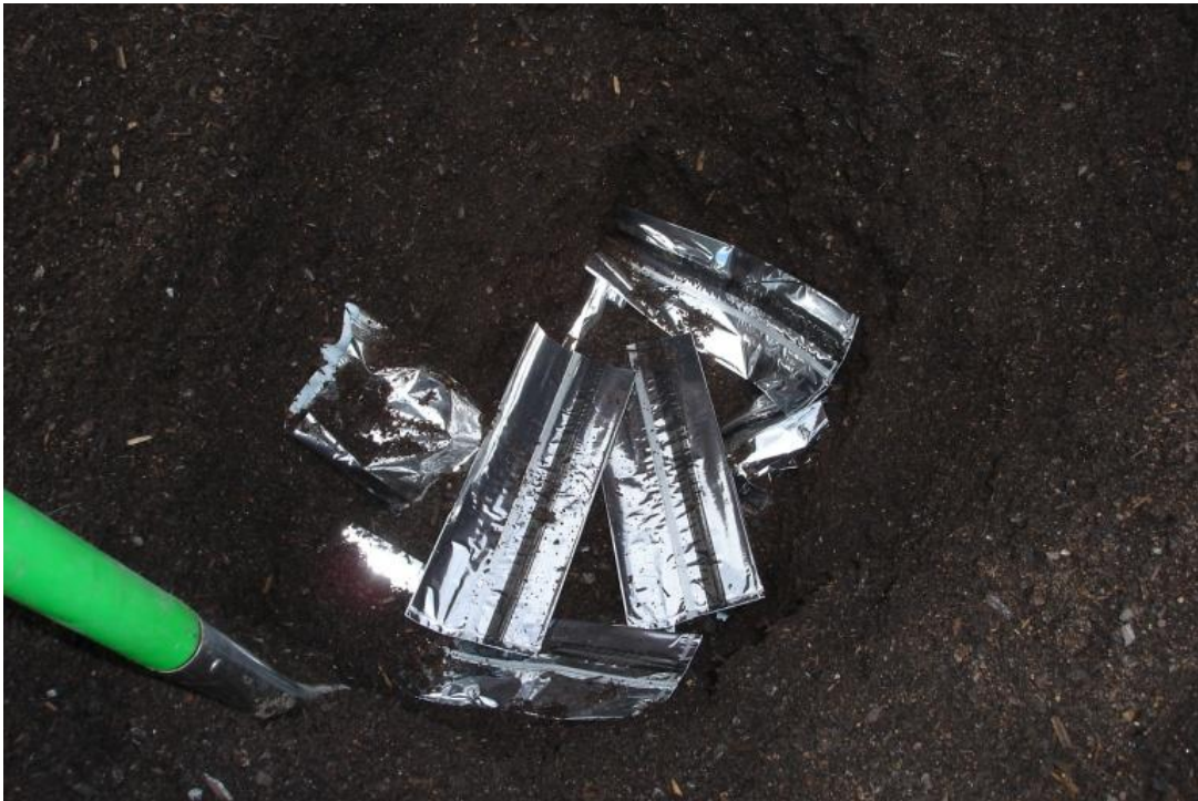
Week 0 - Econic bags being buried.
